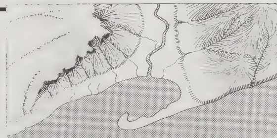
(Above) The hachure method of relief portrayal. (Right) The hypsometric (or layer tint) method.
